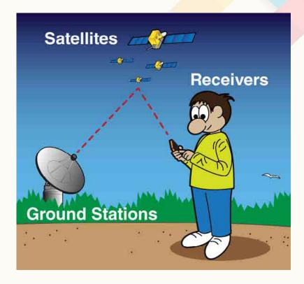
The Global Positioning System (GPS) is made up of satellites, ground stations, and receivers. Satellites act like the stars in constellations—we know where they are supposed to be at any given time.
